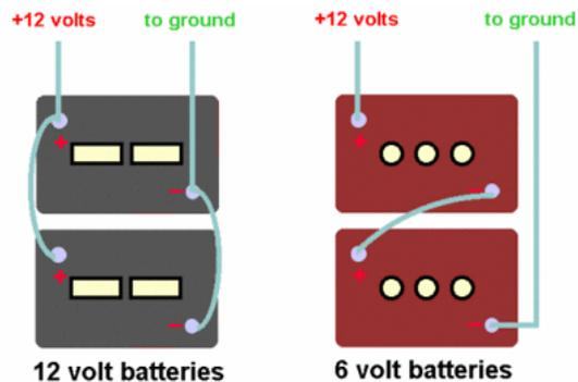
I'll go with the experts one more time. If you are replacing batteries or upgrading and space is not an issue, I'd recommend two 6-volt batteries wired together over single 12-volt batteries. NOTE: When people tell you to put "golf cart" batteries in your RV, they are talking about 6-volt deep cycle batteries wired in "series".
