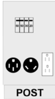
They **should** be labeled with 50, 30, & 20 (or possibly 15 instead of 20), and they **should** be labeled to tell you which position is "off" and which position is "on".
