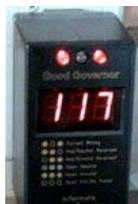
With it, you can test the wiring AND the voltage BEFORE you plug in. However, the Good Governor cannot continuously monitor voltage and it won't prevent electrical voltage drops or surges. Such drops or surges can damage your expensive appliances and electronics.
